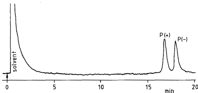
Figure 12 Separation of Tabun enantiomers on an OV-101/Ni(HFB-1R-Cam) 2 complexation column.
